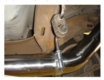
Re-use factory 15mm hardware for the catalytic converter connection.
