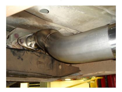
Next insert the axle crossover pipe, and rotate into position ensuring proper clearance for the shock, crossmember, and gas tank. \* Note: Some applications will require minor trimming to the plastic gas tank cover.
