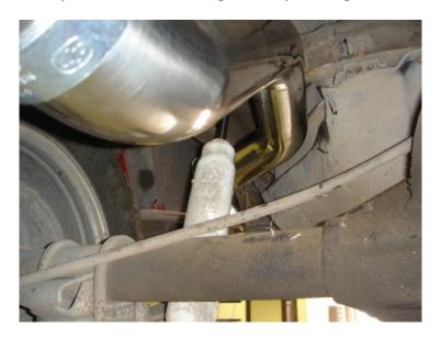
Next, the turndown tailpipe section will slide over the axle pipe, and tighten with the 3" exhaust clamp. This clamp also serves as the second and final hanger. Use the provided clamp and hanger to support the pipe and connect to the factory hanger location. \* Note: Loosen (2) 15mm hanger bolts and flip bracket 180 degrees so it locates further forward, then retighten.
